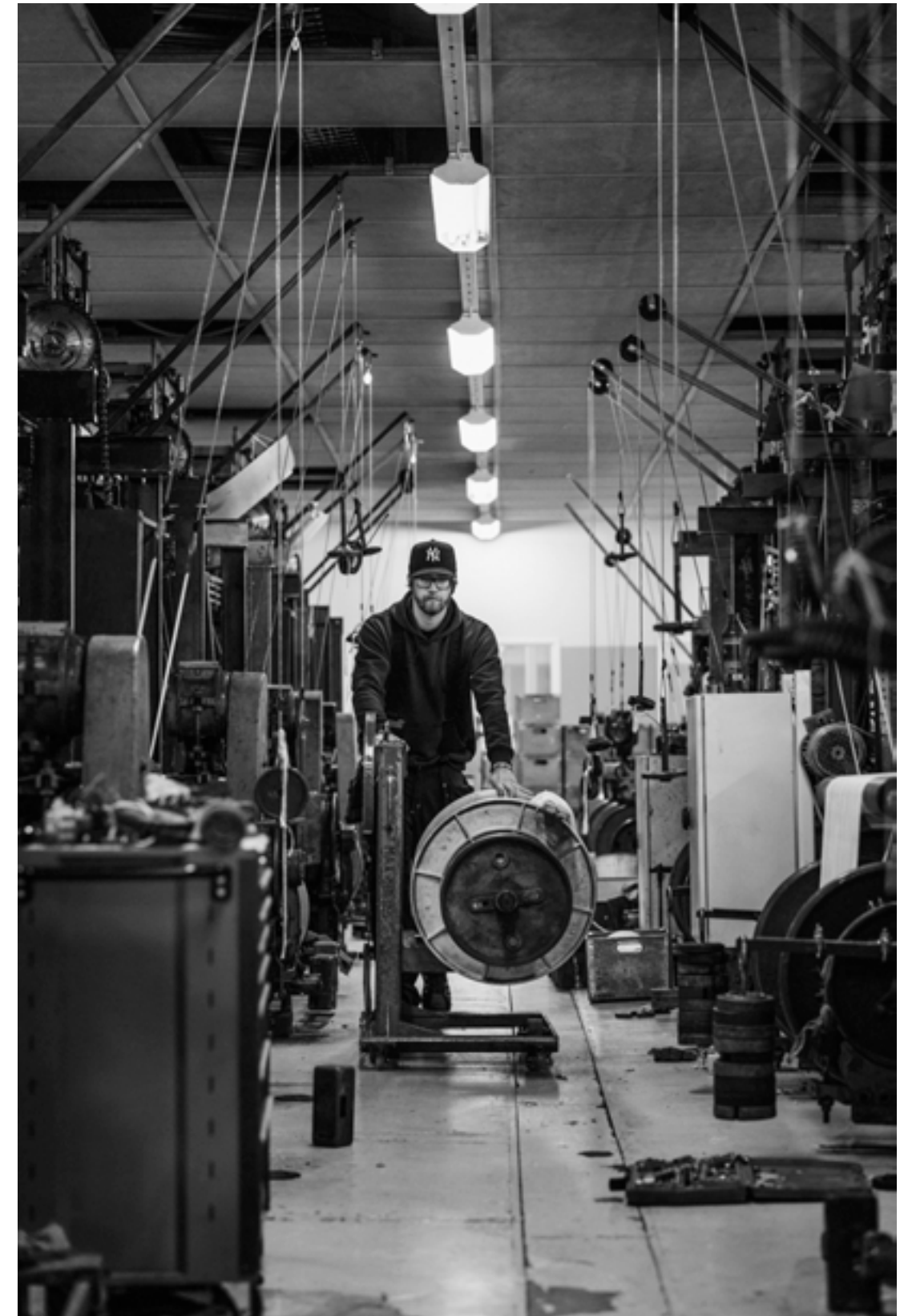
Weaving master Kim changing the warp boom on a loom at our local weaving mill in Sweden.
